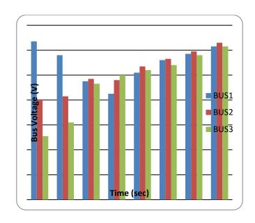
Figure 3: Bus voltages without STATCOM
